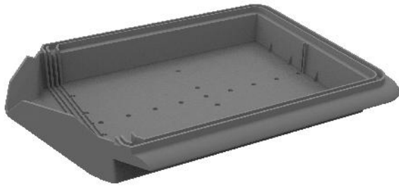
Tray (1) Note the three slots for the baffles.
