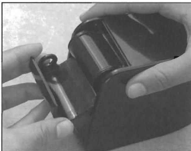
**5** With the end ring of the cassette properly fitted against the light trap of the loader, close the door. Insert the crank, which engages the patented automatic lock and prevents film compartment from opening. For the first few rolls loaded, keep loader on its side while winding to prevent scratches on film base.
