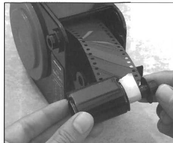
**3** Slide cassette case over spool, with film extending through felt light trap.
