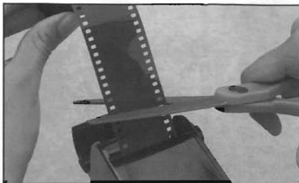
**7** Next, remove the crank from the loader, open the door and take out the cassette. Pull an additional 3-1/2" of the film from the loader for use as a leader when loading the film in the camera. Cut off the film from the bulk roll between the sprocket holes.
