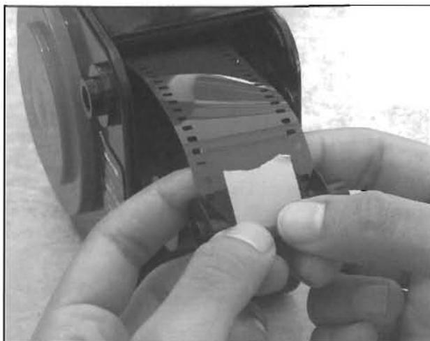
**2** Place end of film against the spool, press one end of tape on top of film and the other end wrap around the spool and tape to the underside of the film. The tape is now looped around the spool and the ends attached to both sides of the film.
