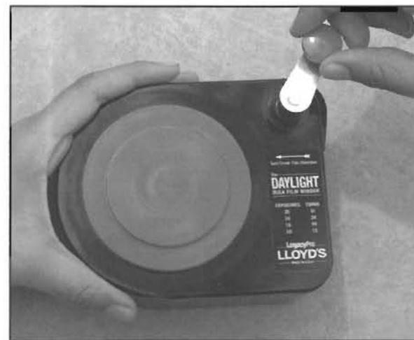
**6** Hold the loader with the left hand and with your right hand wind the correct number of turns for the exposures you want in the cassette. The turns will vary somewhat with different spool diameters, as some are bigger than others. Generally, 36 exposures in a cassette equals 30 turns of the crank.
