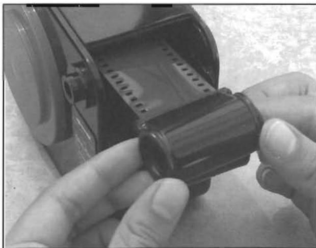
**4** When using reloadable metal cassettes, put an end ring over the spool end and snap over the edges of the spool. Pull down lightly on the end and it will snap into place. Give the ring about 1/8 of a turn to see that it is properly seated into the groove.
