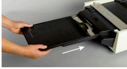
Slide the holder forward, with light downward pressure to feed it through the spring loaded tray.
