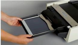
Before loading the negative holder, always check that the sheet is lying flat. If the sheet curls up too much, it can get stuck or misalign during processing.
