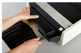
Insert the transparent positive sheet into the tray, with with the chemical pod leading into the tray and the pod facing up.
