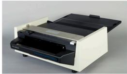
Check your rollers before processing each sheet of film. The rollers can be lifted out for inspection by unlocking the two latches on either side of the metal cover.
