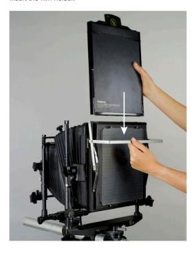
Before making the exposure pull the dark slide straight up. Lift the dark slide up until the bottom blue line is just showing. When pulling the dark slide, do not pull on the negative itself; the paper tongue with the yellow arrow. Shoot your photo!
